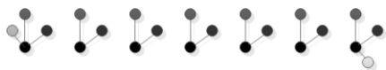
Figure 11. Partial assembly connectivity graph representing merged beam nodes (vertices) connecting to two separate sets of panel nodes (medium and dark grey). Beam end nodes connect to an additional panel component at the corner vertices of a box.
