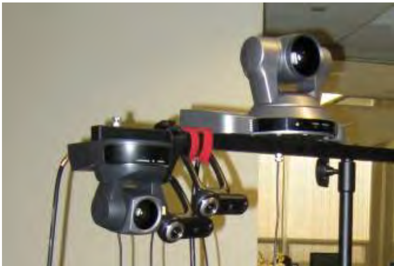
Figure 20: Cameras Affixed to Adjustable-Height Arm
