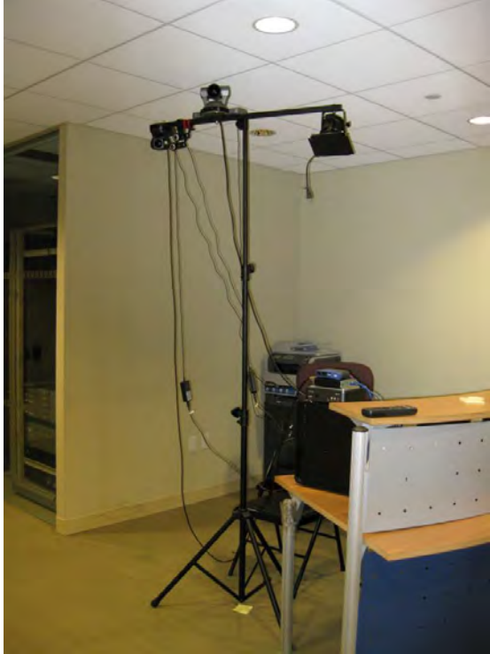
Figure 23: Cameras at Height of 8.0'
