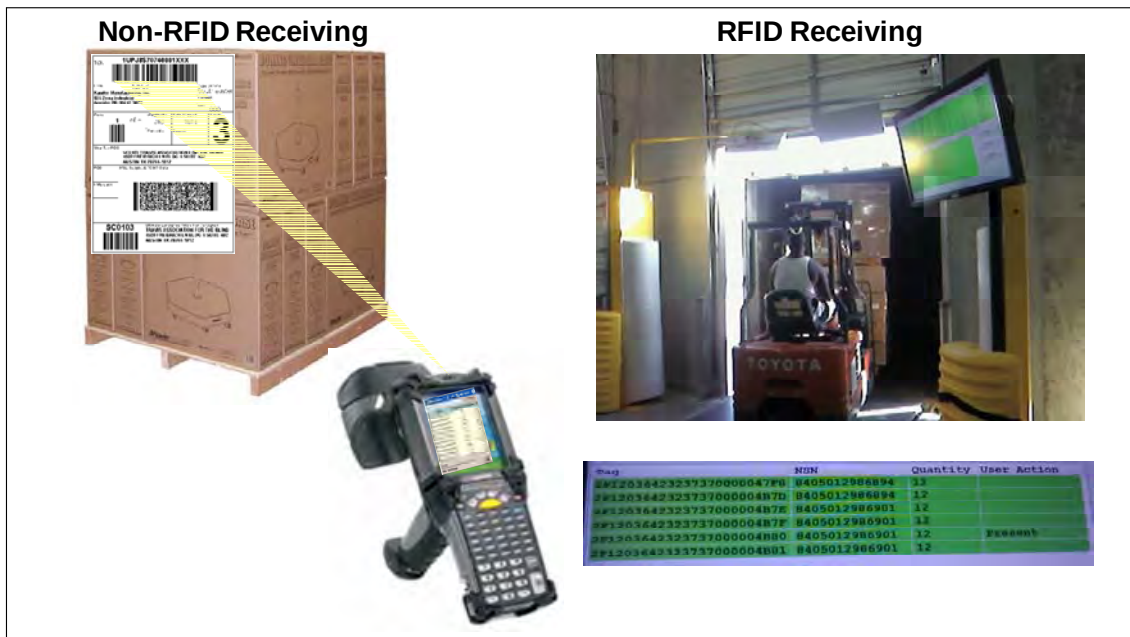
Figure 3.4.1: 3PL Receiving Utilizing Bar Code and RFID Portal Scanning
