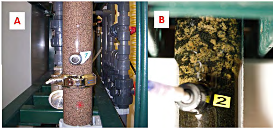
Fig. 2. (A) Left: biomass in the FBR on Day 47. Type I methanotrophic bacteria dominated the biofilm appeared pink in color. (B) Right: biofilms on Day 252 with Type II methanotrophic bacteria as dominant species. The biomass appeared tan in color and formed larger clumps.
