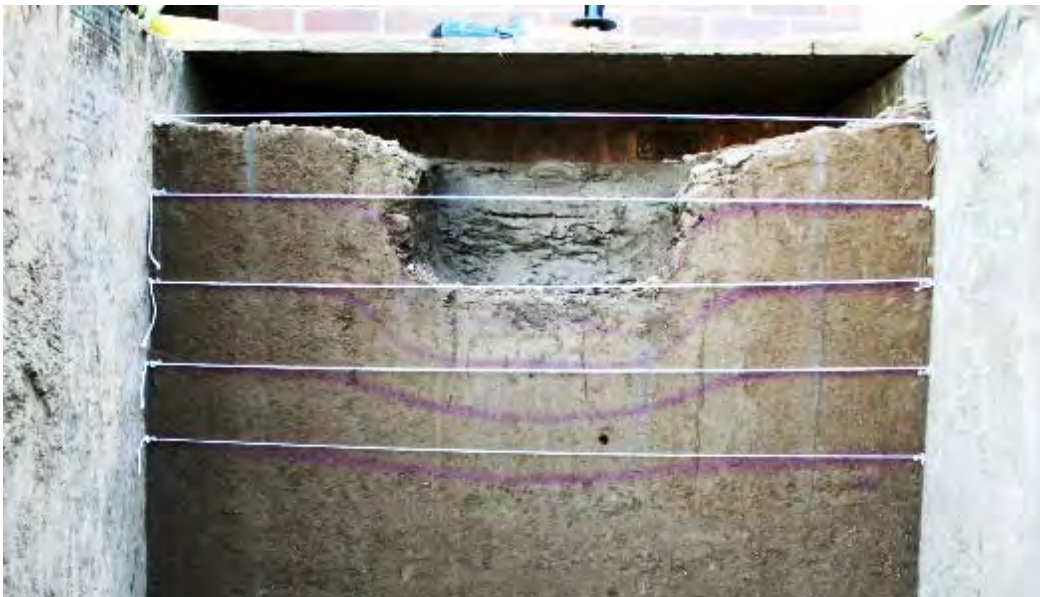
Figure 5. Example of Visible Deformation Made Possible by the Addition of Dyed Soil Layers
