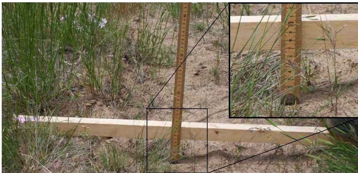
Figure 60. Rut Left in Previously Undisturbed Area by M1A1 Tank After Four Passes
