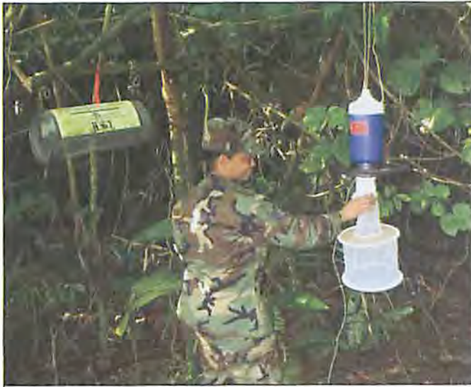
Figure 2. CDC light trap used to collect mosquitoes, including Anopheles sinensis , from a housing area in Andersen AFB, Guam, December 2007.
