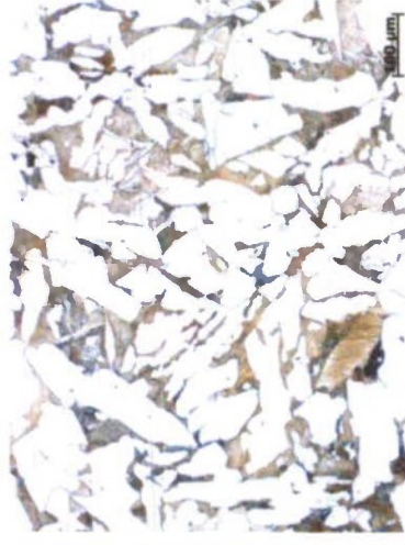
1030 as-cast with NbO addition
