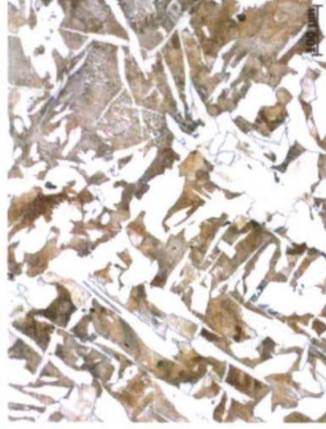
1030 as-cast and no additions
