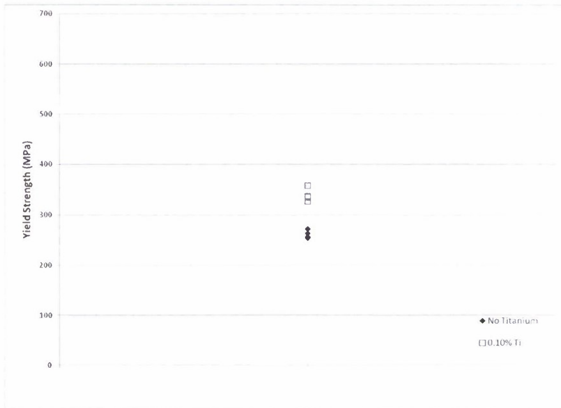
Figure 17 Yields strength for the tensile bars made from cast plates.
