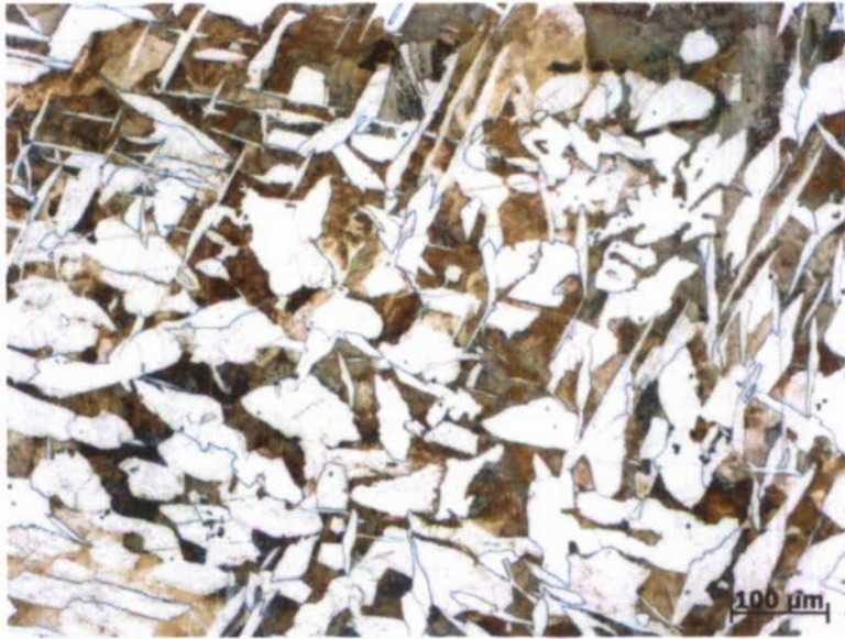
Figure 27 As-cast 1030 with 0.1% misch metal addition micrograph.
