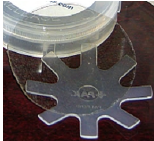
Figure 2. Picture of a 2 inch AlN on-axis ( c -axis) wafer with \sim 85\% usable area. The wafer was cut from a single crystal boule. (Courtesy of L. Schowalter, CIS, USA.)
