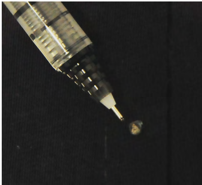
(b) Dielectric failure point with a 0.5 mm tipped pen for perspective
