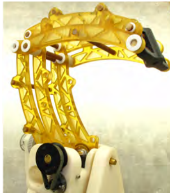
Fig. 7. Photograph of the remote center of motion (RCM) linkage portion of the DBS insertion mechanism that couple to the above-mentioned translational motion base.
