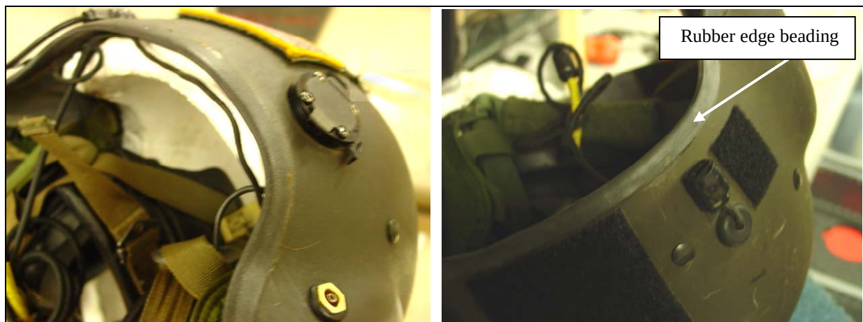
Figure 2. HGU-56/P aviation helmet without beading (left) and with beading (right).
