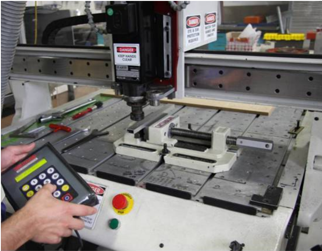
Figure 26: Adjusting the X-Y position of the router cutter bed
