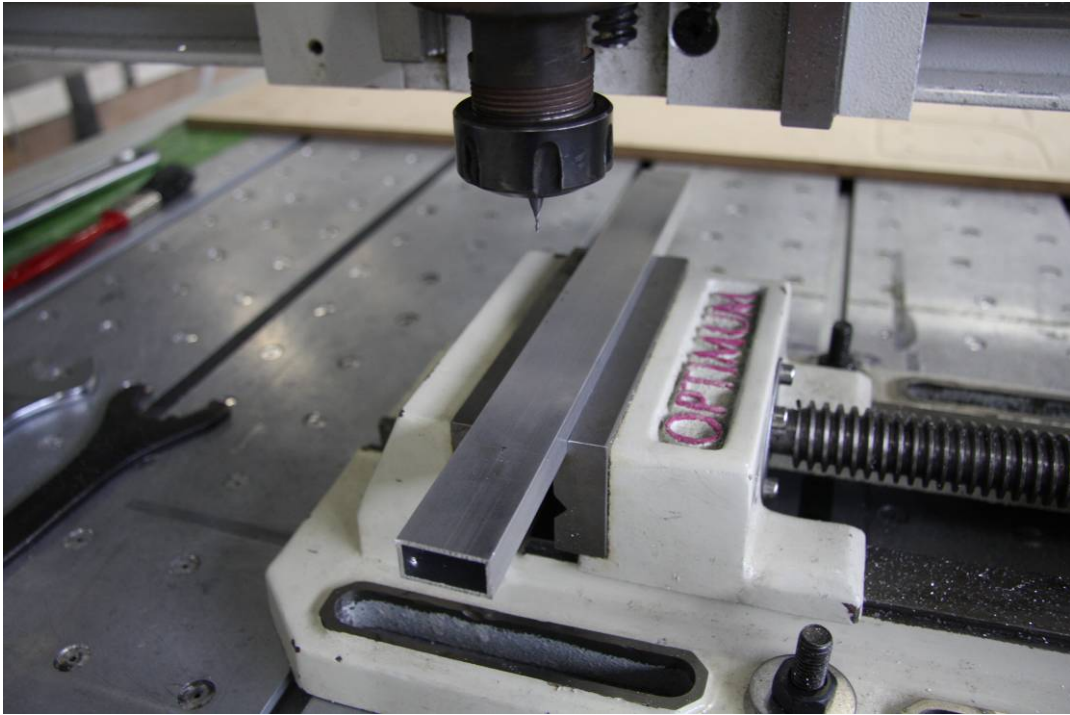
Figure 25: An aluminium waveguide clamped in vice on the Multicam M-I CNC Router bed
