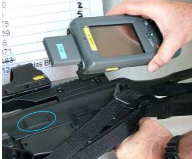
Figure 19. An RFID Tag on the G36 Assault Rifle in the U.K. Police Force. 79
