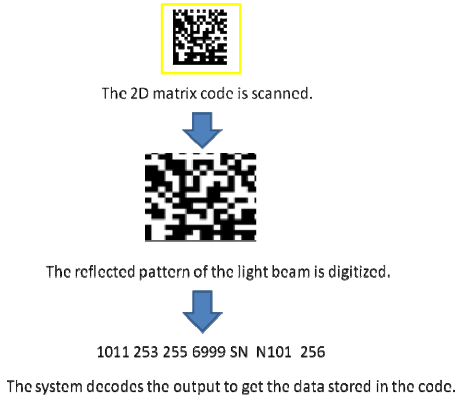
Figure 9. Steps in Reading and Decoding a 2D Matrix Code.
