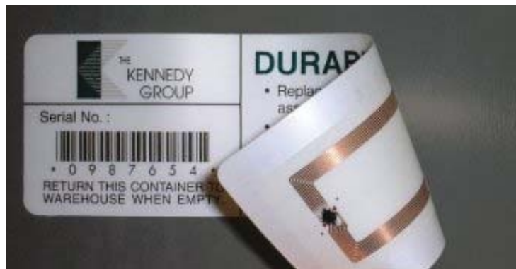
Figure 4. Passive RFID Tag Embedded in Label. 17
