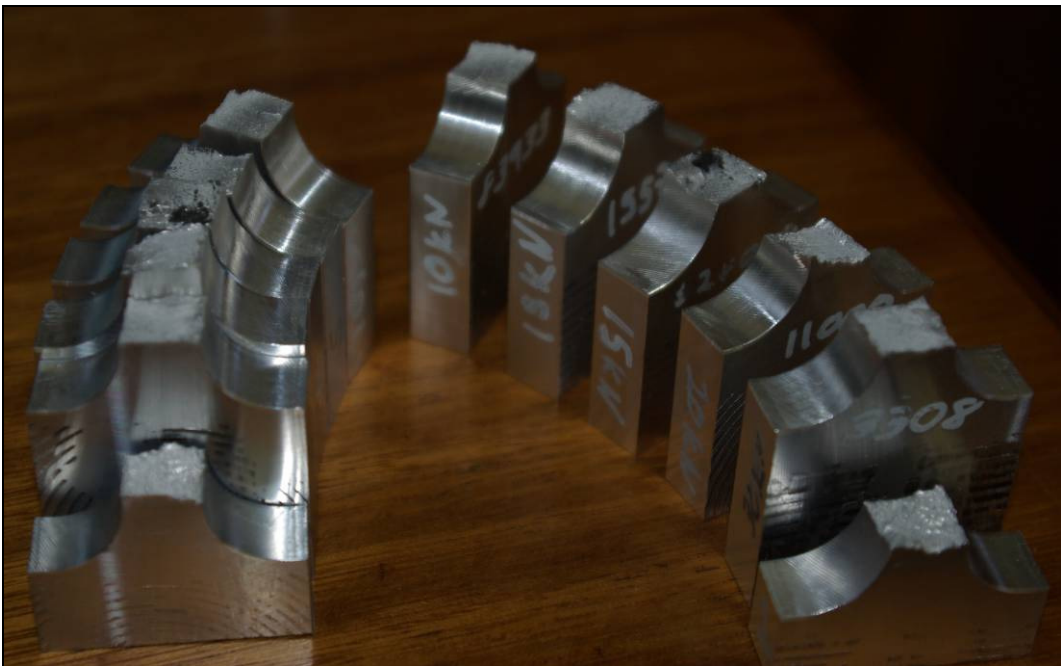
Figure 3 – Fatigue test specimens after failure
