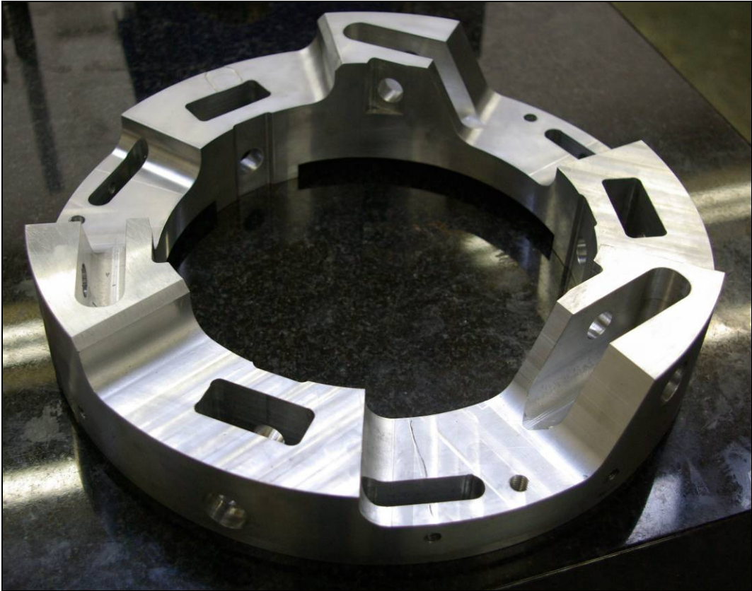
Figure 10 – Manufactured improved flange
