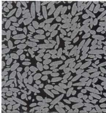
Figure 2.8. The cross-section of the voxel pack after thresholding.
