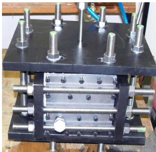
Figure 11. Generator showing Bracing Rods & Clamping Bolts
