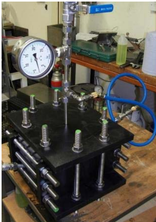
Figure 12. Generator Undergoing Preliminary Pressurization to 3 Bar
