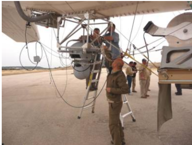
Figure 3. Installation of the equipment on the PGSS aerostat gondola.
