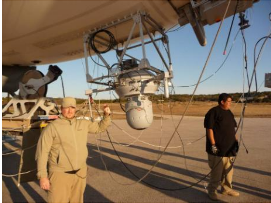
Figure 8. High-gain repeater antenna mounted on the PGSS camera gondola.
