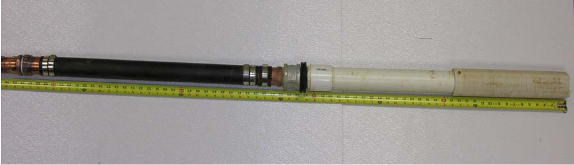
Figure 53b. Pneumatic source assembly consisting of a PVC screen interval, PVC blank, wafer packer, and inflation packer.
