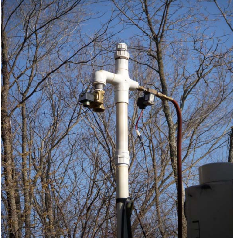
Figure 5b. Pneumatic pressure manifold with servo-controlled valves.
