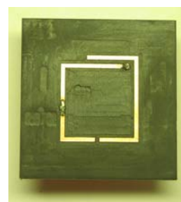
Fig. 1: Pattern reconfigurable antenna. Depending upon switch location, patterns can range from broadside to endfire with linear polarized beams.
