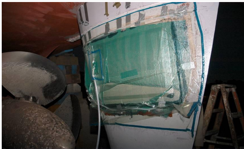
Vacuum Bag to Hold Section in Place for Cure
