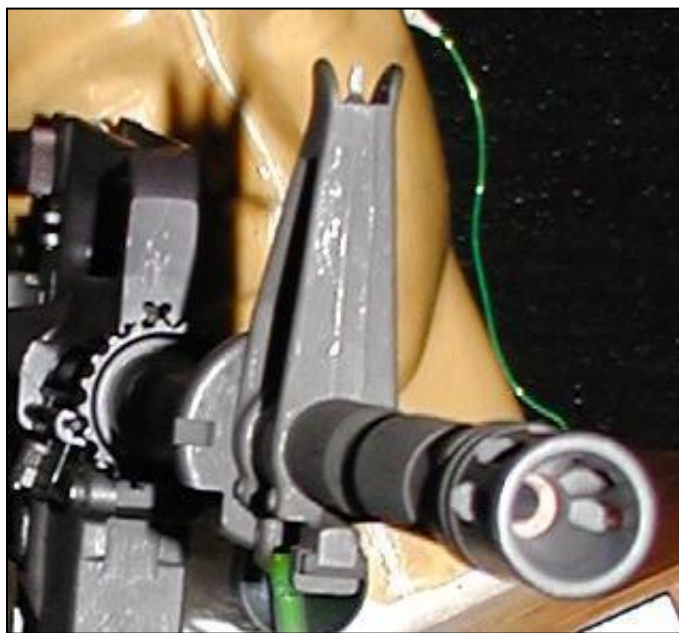
Figure 30. Muzzle compensator with asymmetric venting.
