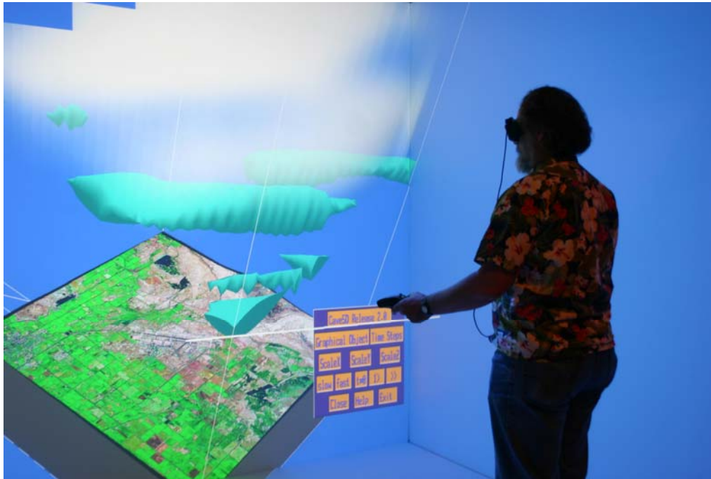
Figure 10. Visualization of the real-time forecasts of turbulence and cloudiness over the runway for the Fallon NAS in the CAVE (Cave Automatic Virtual Environment). A person in the CAVE can interactively probe forecast results with respect to various model domains, times, and forecasted parameters. For this visualization, white represents cloud, while cyan represents areas of high turbulence kinetic energy.
