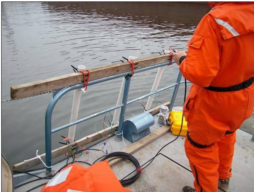
Figure 5. Installation of probe frame on test vessel.
