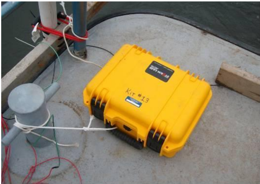
Figure 8. GPS receiver and logger on aft deck of test vessel.
