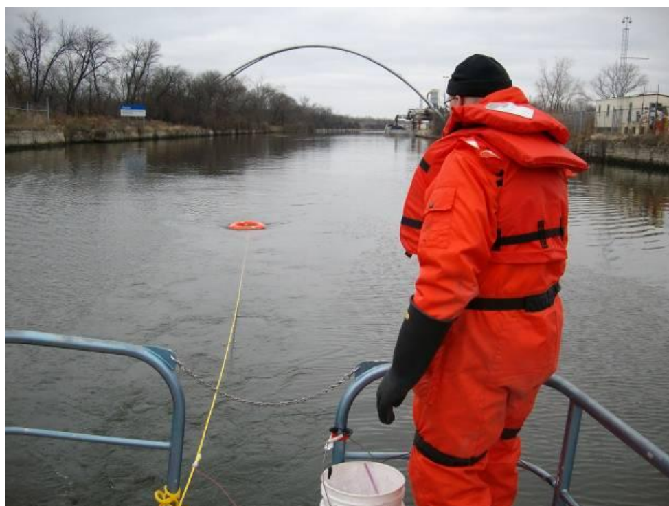
Figure 16. Test vessel towing life ring and simulated PIW with polypropylene recovery line.
