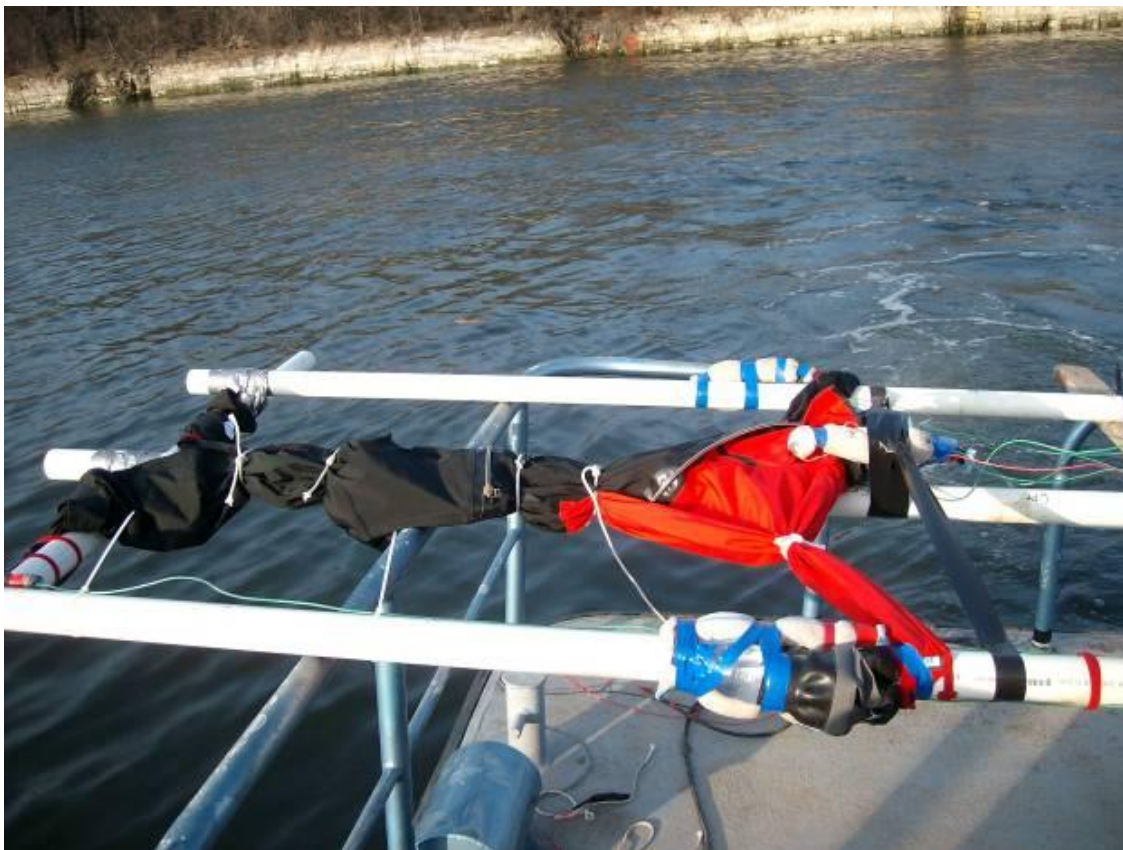
Figure 14. Dry suit test apparatus mounted to sensor array frame.
