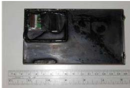
Figure 2. An IBM 4758-001 part potted in urethane, showing membrane and interior.
