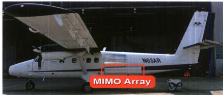
Figure 8. MIMO flat panel array mounted on the side of the Twin Otter aircraft.
