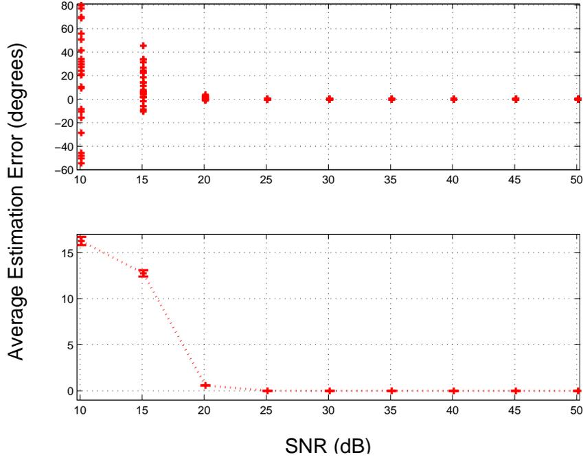
Figure 4.41: Azimuth estimation error vs. SNR for an  $f_c = 11$  MHz incident signal using  $N_A = 8$  feed points to synthesize a cube antenna pattern. Top: Average estimation error of 24 azimuth angles based on 200 Monte Carlo iterations. Bottom: Estimation error averaged over 200 Monte Carlo iterations and 24 azimuth angles with 95% confidence intervals.
