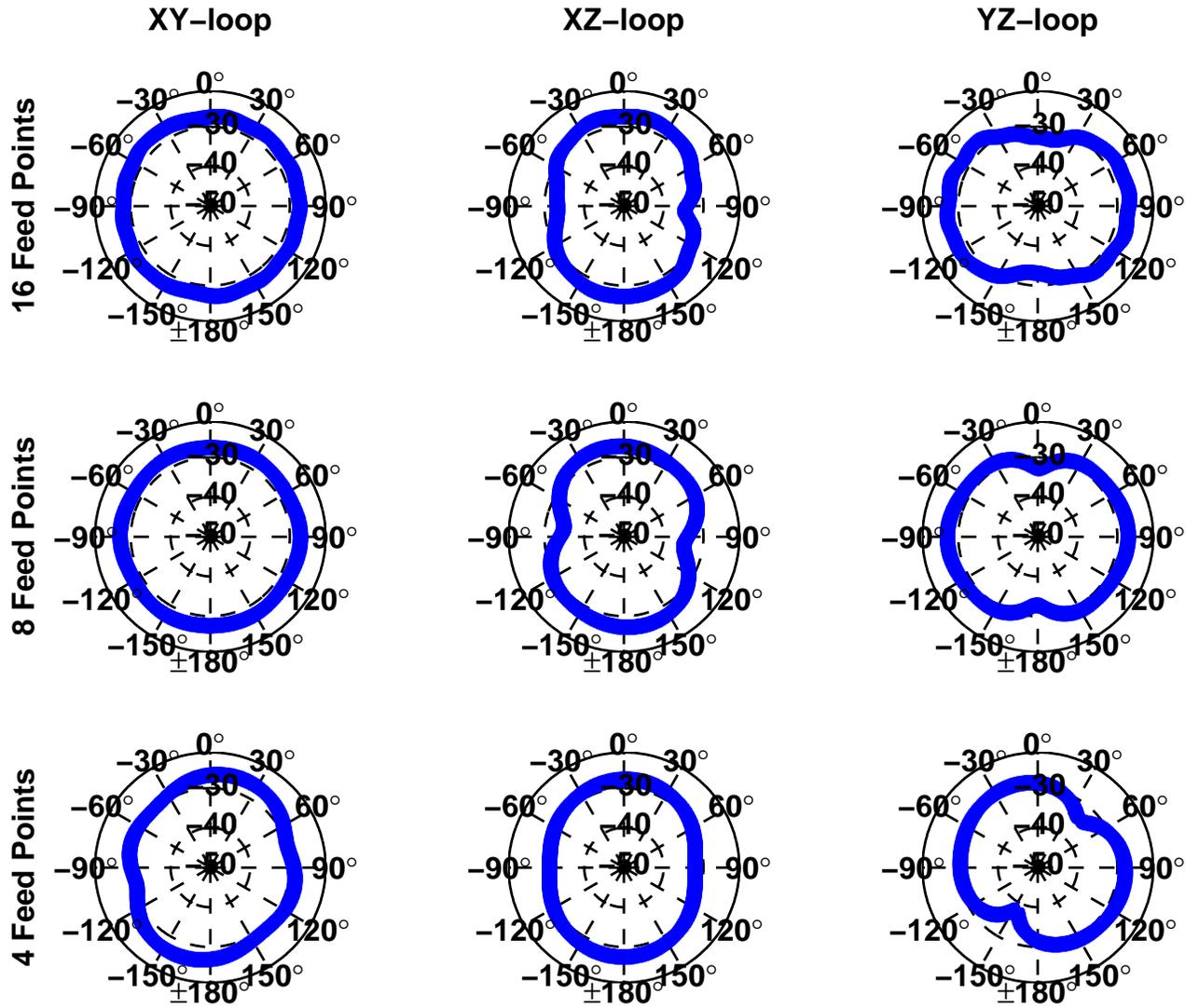
Figure A.4:  $f_c = 11$  MHz synthesized cube antenna patterns. Each row contains all 3 loops for linear combinations of  $N_A = 16$ ,  $N_A = 8$ , and  $N_A = 4$  feed points.
