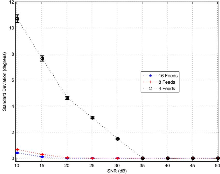
Figure 4.21: Standard deviation of azimuth estimation error vs. SNR for an  $f_c = 11$  MHz incident signal. Standard deviation based on average estimation error over 200 iterations of 24 azimuth angles.
