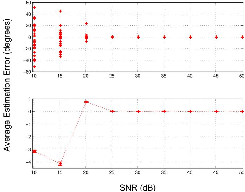
Figure 4.30: Azimuth estimation error vs. SNR for a  $f_c = 4$  MHz incident signal using  $N_A = 8$  feed points to synthesize a cube antenna pattern. Top: Average estimation error of 24 azimuth angles based on 200 Monte Carlo iterations. Bottom: Estimation error averaged over 200 Monte Carlo iterations and 24 azimuth angles with 95% confidence intervals.
