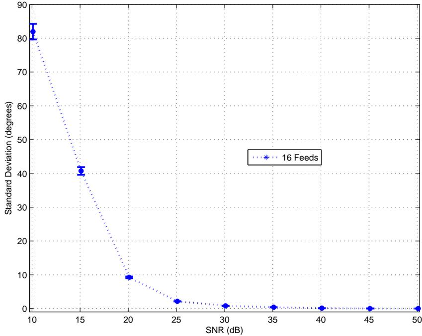
Figure 4.39: Standard deviation of AOA estimation error vs. SNR for an  $f_c = 11$  MHz incident signal with 95% confidence intervals using  $N_A = 16$  feed points to synthesize a cube antenna pattern.
