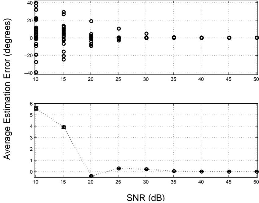
Figure 4.33: Azimuth estimation error vs. SNR for a  $f_c = 4$  MHz incident signal using  $N_A = 4$  feed points to synthesize a cube antenna pattern. Top: Average estimation error of 24 azimuth angles based on 200 Monte Carlo iterations. Bottom: Estimation error averaged over 200 Monte Carlo iterations and 24 azimuth angles with 95% confidence intervals.
