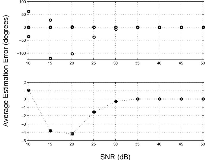
Figure 4.18: Azimuth estimation error vs. SNR for an  $f_c = 11$  MHz incident signal and  $N_A = 4$  individual feed points. Top: Average estimation error of 24 azimuth angles based on 200 Monte Carlo iterations. Bottom: Estimation error averaged over 200 Monte Carlo iterations and 24 azimuth angles with 95% confidence intervals.
