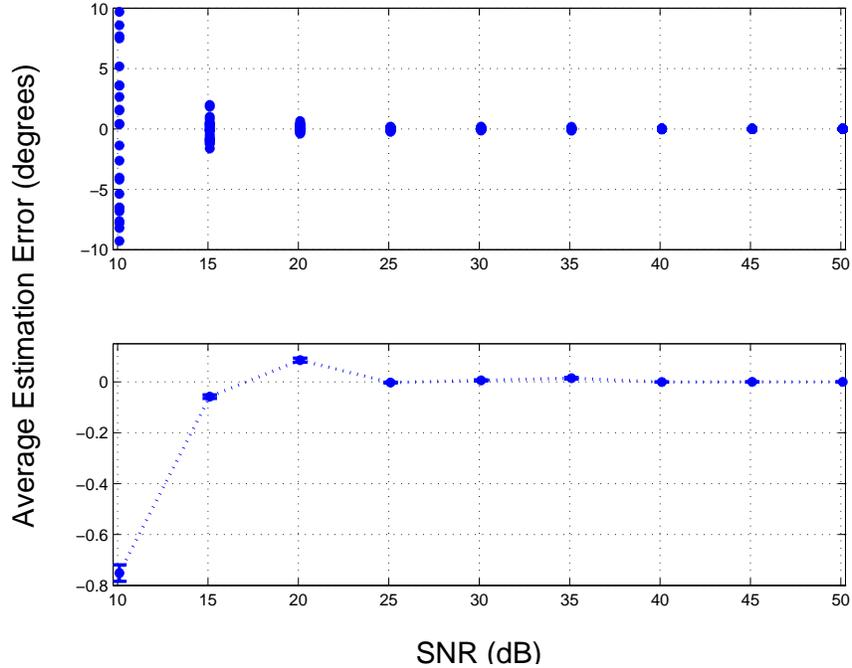
Figure 4.27: Azimuth estimation error vs. SNR for a  $f_c = 4$  MHz incident signal using  $N_A = 16$  feed points to synthesize a cube antenna pattern. Top: Average estimation error of 24 azimuth angles based on 200 Monte Carlo iterations. Bottom: Estimation error averaged over 200 Monte Carlo iterations and 24 azimuth angles with 95% confidence intervals.
