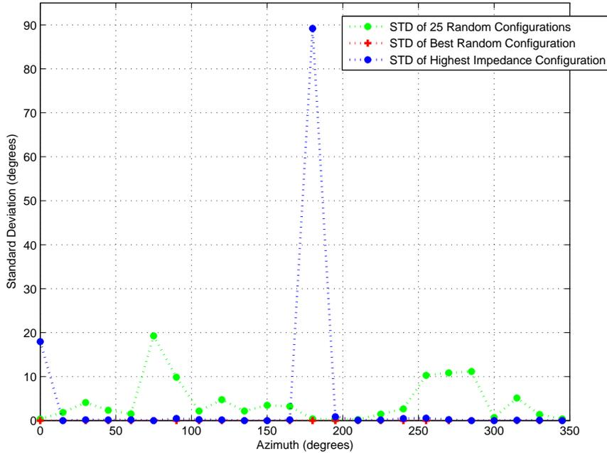
Figure 4.26: Standard deviation vs. Azimuth. Performance of best  $N_A = 4$  random feed point configuration compared to the mean standard deviation of 25 random configurations and  $N_A = 4$  feed point configuration with highest input impedance. Results based on an  $f_c = 11$  MHz incident signal with  $SNR = 20$  dB.
