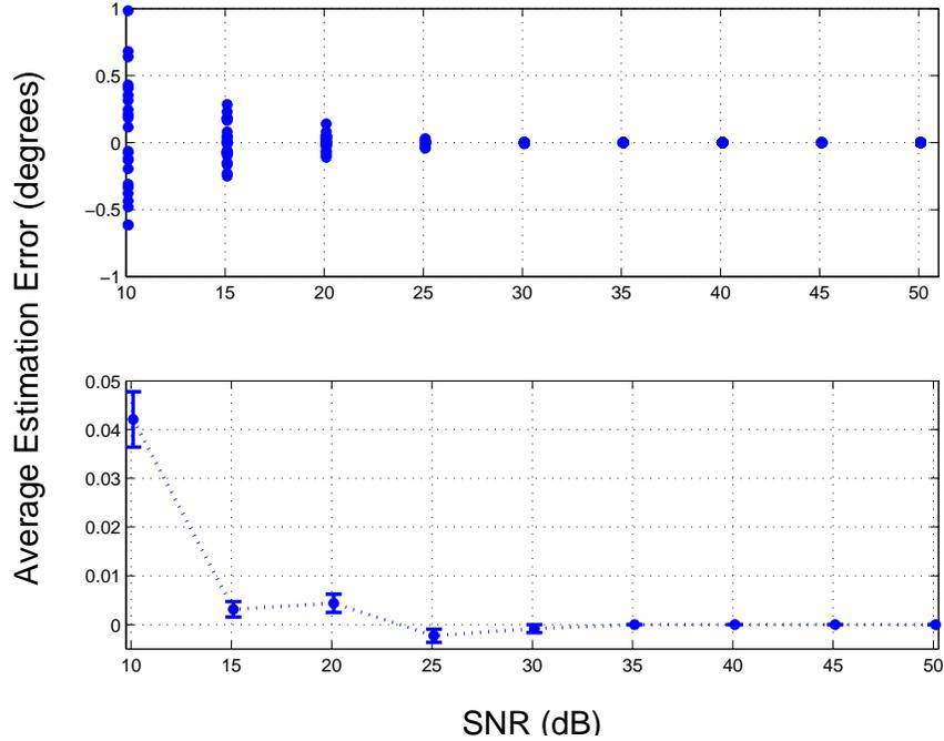
Figure 4.1: Azimuth estimation error vs. SNR for a  $f_c = 4$  MHz incident signal and  $N_A = 16$  individual feed points. Top: Average estimation error of 24 azimuth angles based on 200 Monte Carlo iterations. Bottom: Estimation error averaged over 200 Monte Carlo iterations and 24 azimuth angles with 95% confidence intervals.
