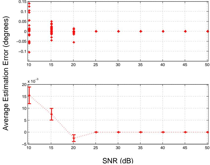
Figure 4.15: Azimuth estimation error vs. SNR for an  $f_c = 11$  MHz incident signal and  $N_A = 8$  individual feed points. Top: Average estimation error of 24 azimuth angles based on 200 Monte Carlo iterations. Bottom: Estimation error averaged over 200 Monte Carlo iterations and 24 azimuth angles with 95% confidence intervals.
