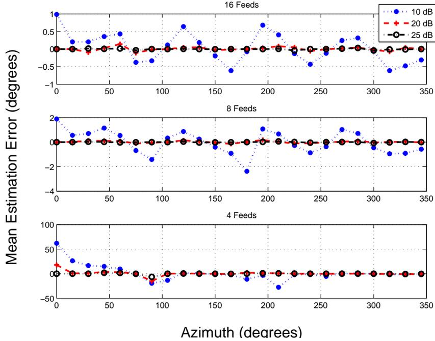
Figure 4.11: Average estimation error vs. SNR for a  $f_c = 4$  MHz incident signal. Results based on multiple values of SNR using combinations of  $N_A = 4$ ,  $N_A = 8$ , and  $N_A = 16$  feed points. NOTE: Error scales (y-axis) are different for each plot.
