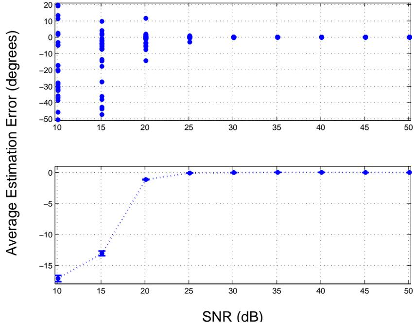
Figure 4.38: Azimuth estimation error vs. SNR for an  $f_c = 11$  MHz incident signal using  $N_A = 16$  feed points to synthesize a cube antenna pattern. Top: Average estimation error of 24 azimuth angles based on 200 Monte Carlo iterations. Bottom: Estimation error averaged over 200 Monte Carlo iterations and 24 azimuth angles with 95% confidence intervals.
