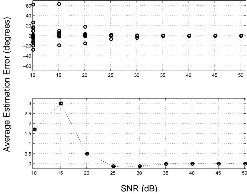
Figure 4.7: Azimuth estimation error vs. SNR for a  $f_c = 4$  MHz incident signal and  $N_A = 4$  individual feed points. Top: Average estimation error of 24 azimuth angles based on 200 Monte Carlo iterations. Bottom: Estimation error averaged over 200 Monte Carlo iterations and 24 azimuth angles with 95% confidence intervals.
