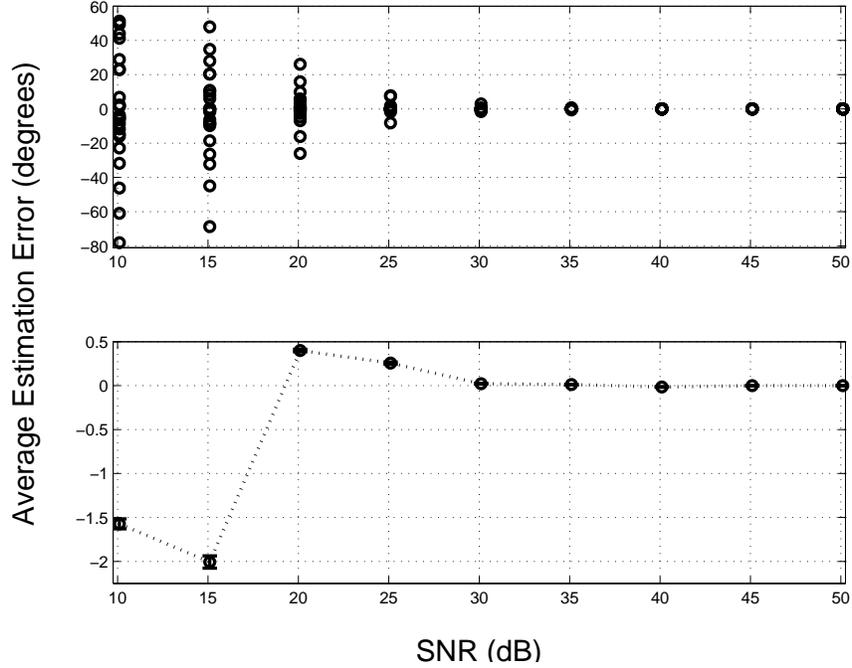
Figure 4.44: Azimuth estimation error vs. SNR for an  $f_c = 11$  MHz incident signal using  $N_A = 4$  feed points to synthesize a cube antenna pattern. Top: Average estimation error of 24 azimuth angles based on 200 Monte Carlo iterations. Bottom: Estimation error averaged over 200 Monte Carlo iterations and 24 azimuth angles with 95% confidence intervals.
