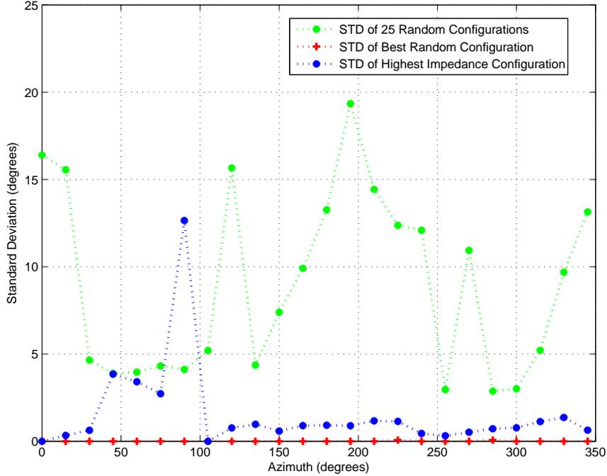
Figure 4.24: Standard deviation vs. Azimuth. Performance of the best  $N_A = 4$  random feed point configuration compared to the mean standard deviation of 25 random configurations and  $N_A = 4$  feed point configuration with highest input impedance. Results based on a  $f_c = 4$  MHz incident signal with  $SNR = 25$  dB.
