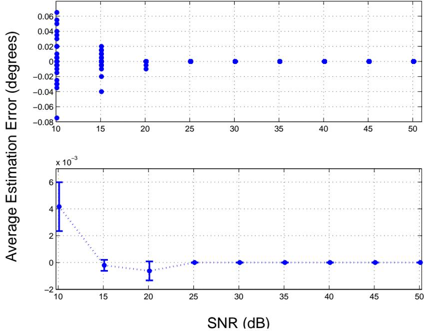
Figure 4.12: Azimuth estimation error vs. SNR for an  $f_c = 11$  MHz incident signal and  $N_A = 16$  individual feed points. Top: Average estimation error of 24 azimuth angles based on 200 Monte Carlo iterations. Bottom: Estimation error averaged over 200 Monte Carlo iterations and 24 azimuth angles with 95% confidence intervals.
