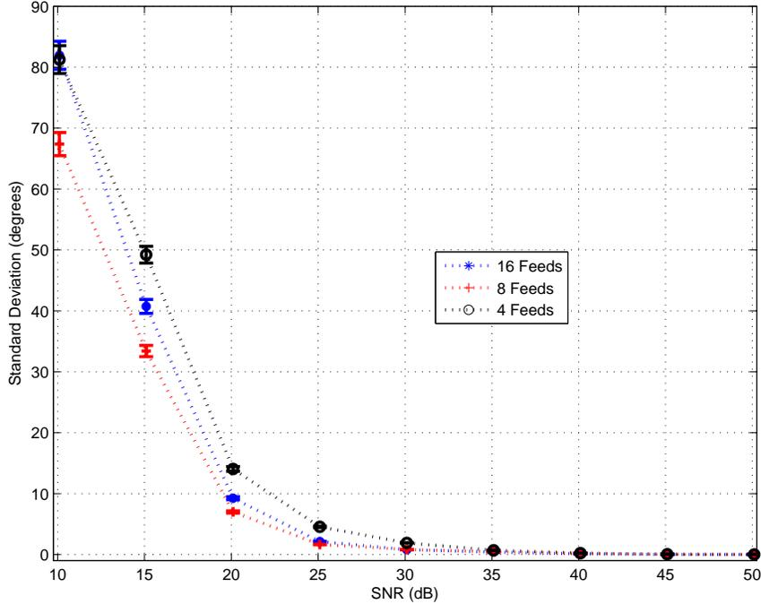
Figure 4.47: Standard deviation of azimuth estimation error vs. SNR for an  $f_c = 11$  MHz incident signal. Standard deviation based on average estimation error over 200 iterations of 24 azimuth angles.
