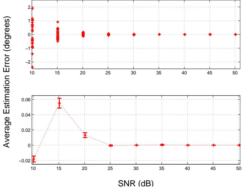
Figure 4.4: Azimuth estimation error vs. SNR for a  $f_c = 4$  MHz incident signal and  $N_A = 8$  individual feed points. Top: Average estimation error of 24 azimuth angles based on 200 Monte Carlo iterations. Bottom: Estimation error averaged over 200 Monte Carlo iterations and 24 azimuth angles with 95% confidence intervals.
