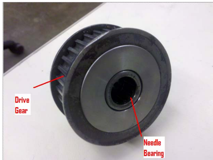
Figure 9: Example of a one-way bearing.
