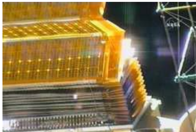
Figure 37. Stowed Solar Panel Being Unfolded for Deployment
