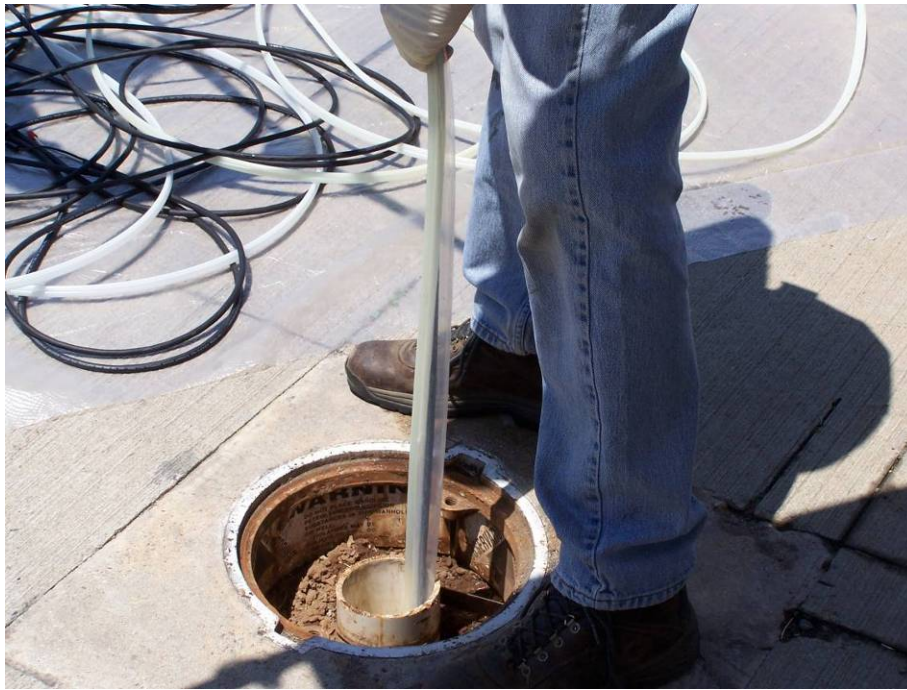
Figure 5-2. Polyethylene covering on electronic trigger line.
