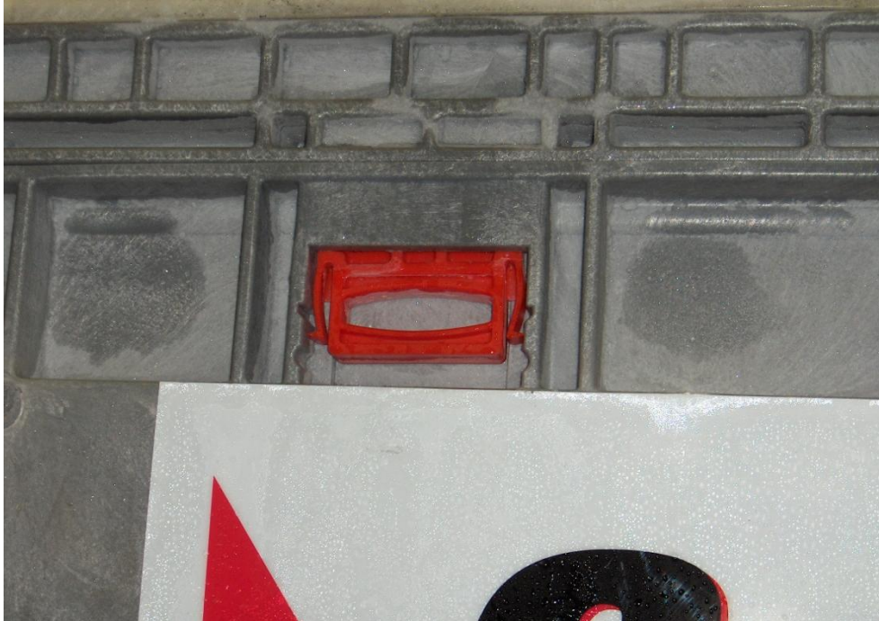
Figure 33. Slippage of latch 2 due to impacts from low temperature rotational drops.
