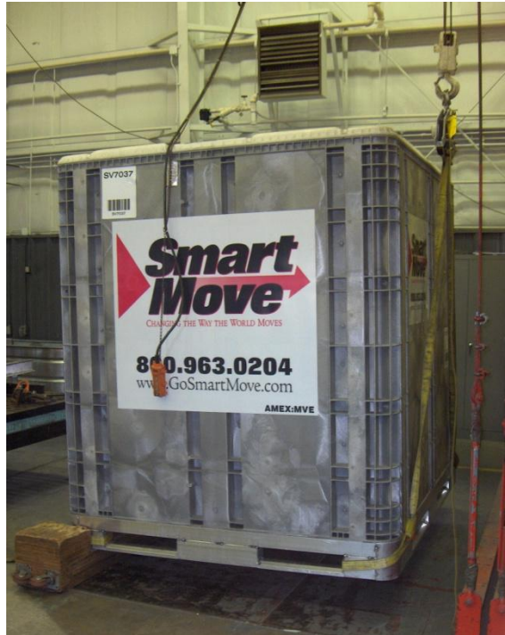
Figure 25. Rotational edgewise drop test, +125°F & 95% RH.
