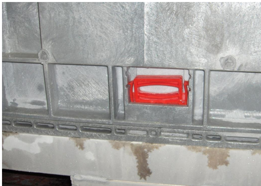
Figure 34. Slippage of latch 6 due to impacts from low temperature rotational drops.
