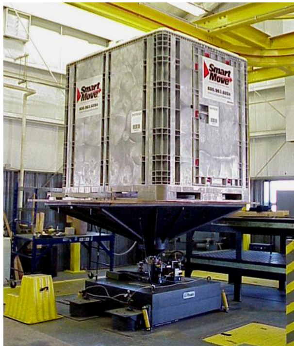
Figure 26. Vibration test, ambient.
