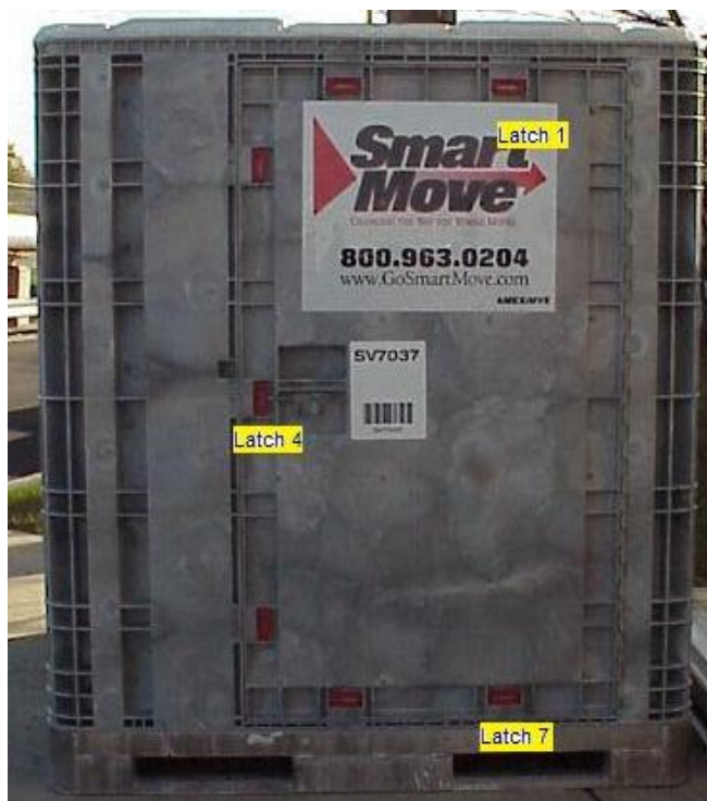
Figure 2. SmartVault container – forward view with counterclockwise door latch numbering system.
