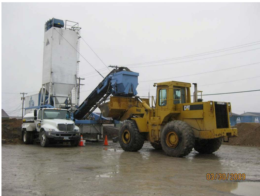
Figure 22. Calibration and trial mixes from continuous pugmill mixer.
