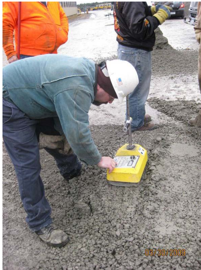
Figure 23. Determining moisture content of trial mix with nuclear gage.
