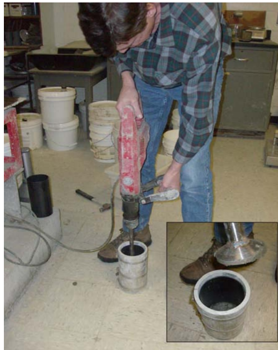
Figure 4. Vibrating hammer with tamper foot (inset) used to compact laboratory test specimens for unconfined compressive strength test.
