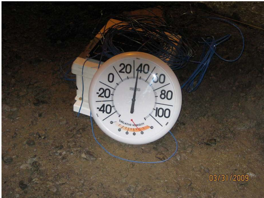
Figure 24. Air temperature reading at start of cold-RCC operation.
