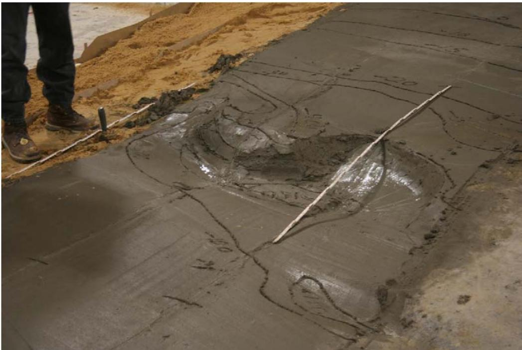
Figure 14. Hand molding Cairn Point bathymetry on the Large-Area Model.
