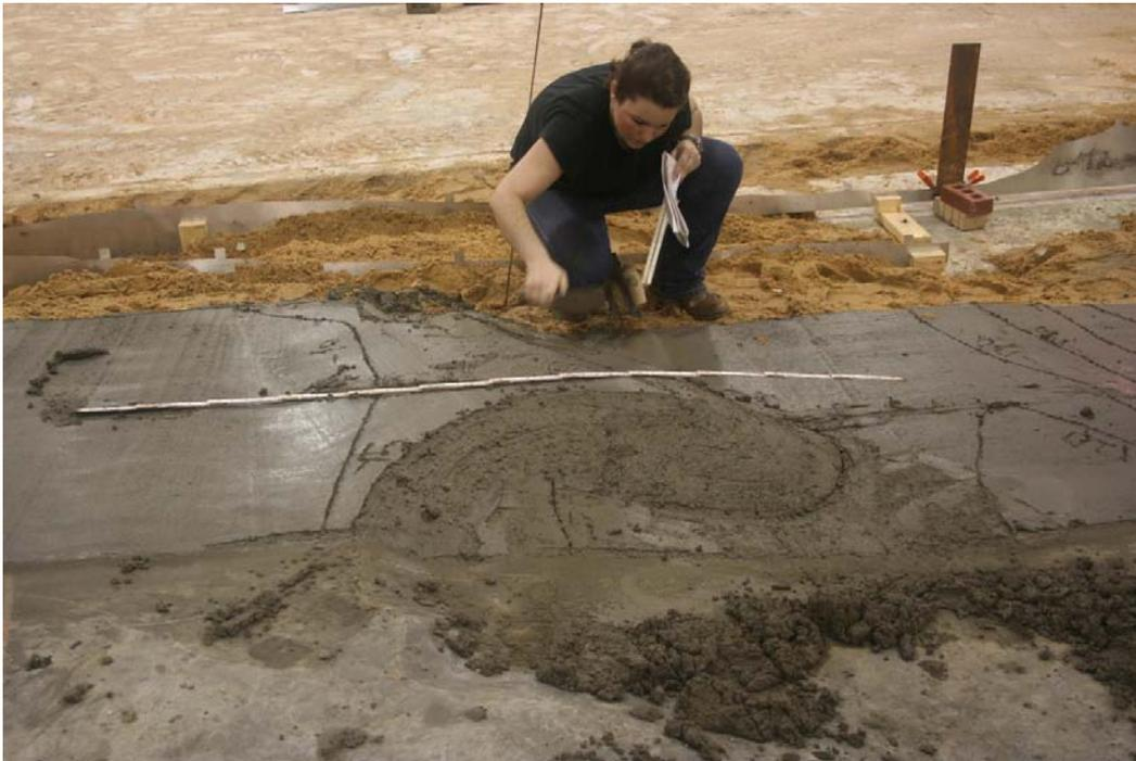
Figure 13. Hand molding bathymetry detail on the Small-Area Model.
