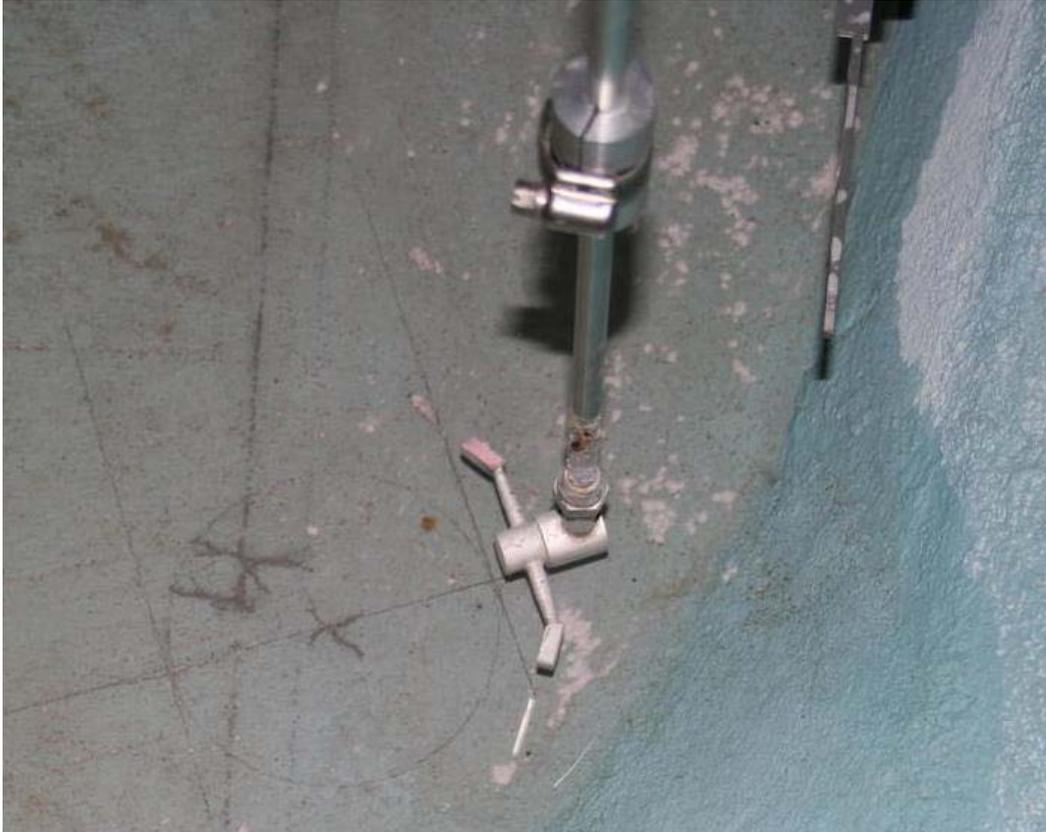
Figure 21. Acoustic Doppler velocimeter probe head.
