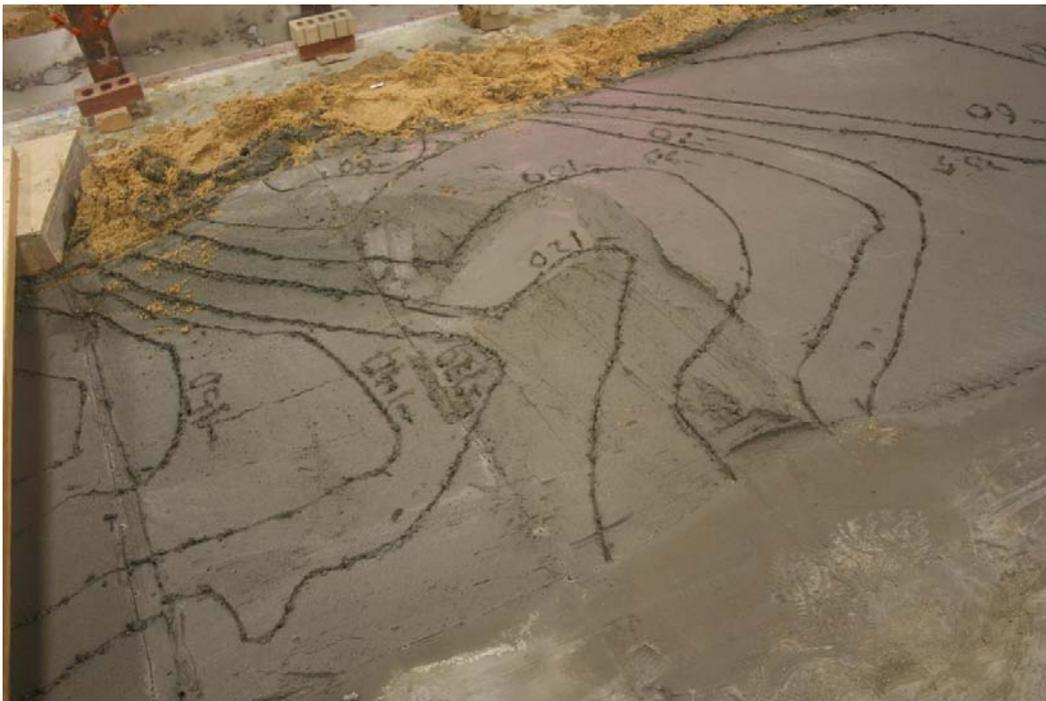
Figure 12. Bathymetry contours sketched on the Small-Area Model.
