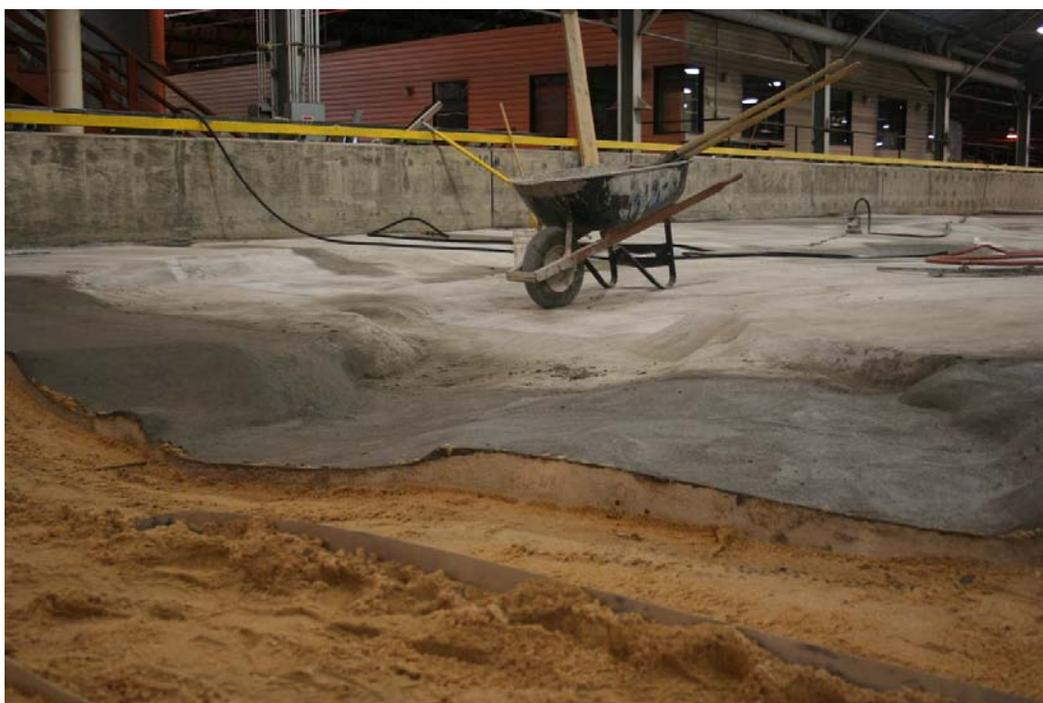
Figure 15. Cairn Point bathymetry detail on the Large-Area Model.
