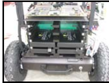
Figure 3: UGV's Hot-Swap Battery Pack.
