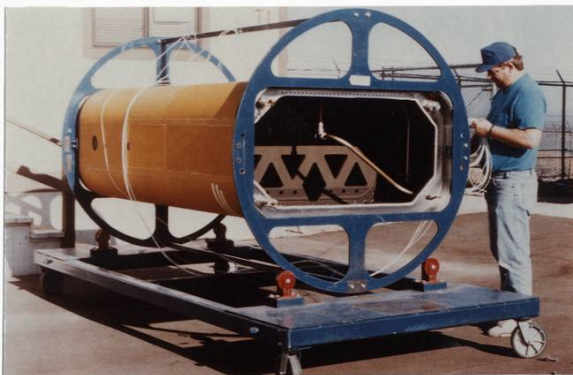
Figure 8. Conformal Cryotank Was Fabricated and Tested at Convair's Rye Canyon Facility
