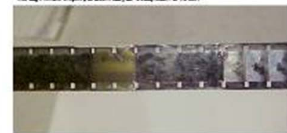
Damage from solvents
