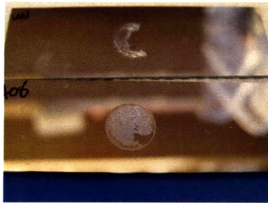
Figure 2-13: Results of adhesion test of pHEMA-co-MAA (top) and A08-modified pHEMA-co-MAA to aluminum-coated slides (bottom).
