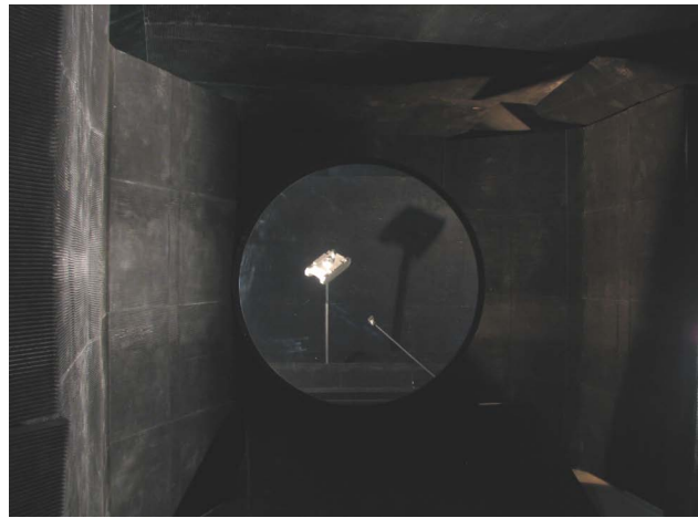
Figure 2 – Primary (Antenna) Mirror in Compact Range with Surrounding Anechoic (Complex Target Simulator (CTS) and In-Scene Dihedral Visible in Reflection)
