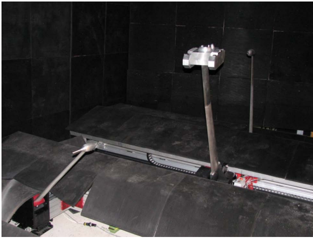
Figure 3 – Front Angled View of Target Positioning System with Calibration Pylon at the Rear (Right), Target Pylon with Adjustable Elevation (Middle), In-Scene Calibration Pylon with Dihedral (Front-Left)
