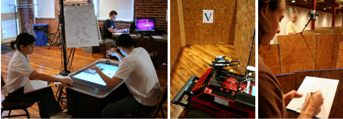
Figure 6-4: The participant is observed using the multi-touch interfaces (left) to search for victim marker using an ATRV-Jr robot (middle) while test administrators (right) record video and written documentation regarding the performance of the run.
