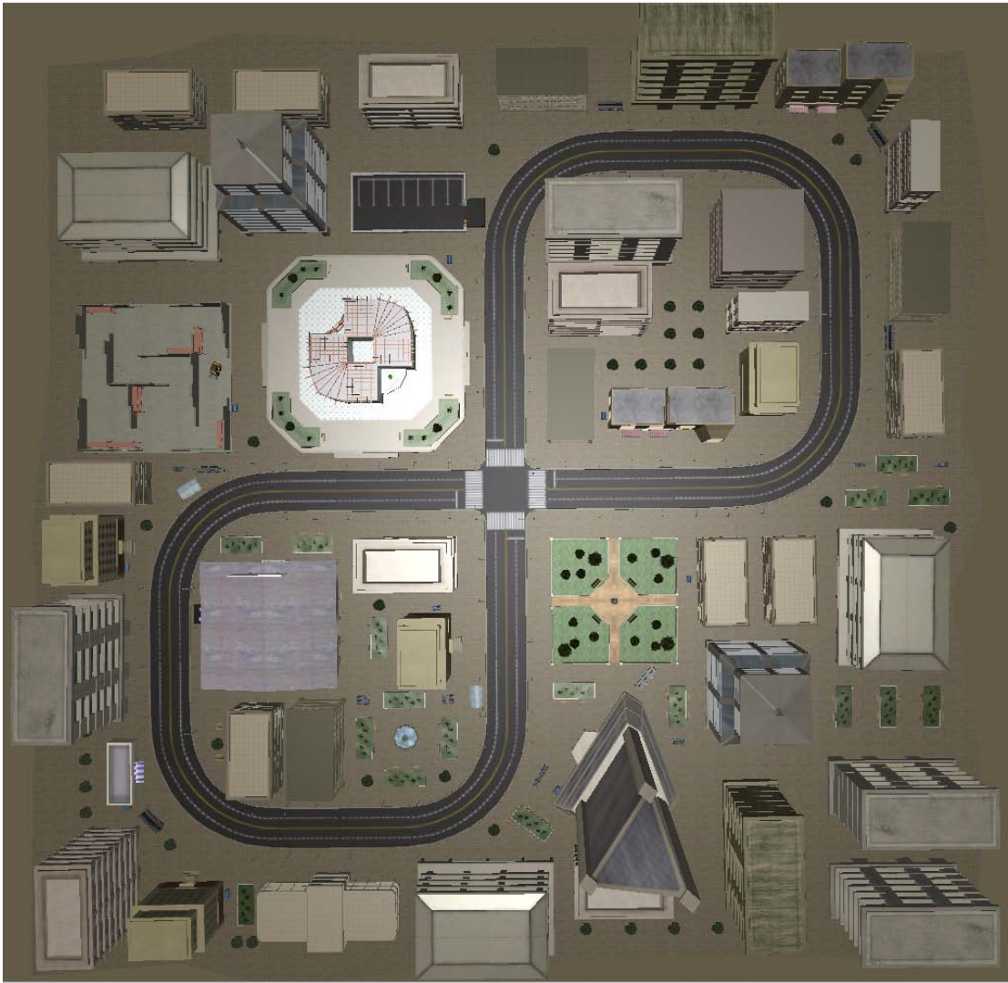
Figure 8-6: An aerial view of the urban simulation environment used to test the gesture based command and control interface. The three dimensional city was approximately 2 acres in area and used realistic hardware-accelerated physics for robot movement and interaction with the environment.
