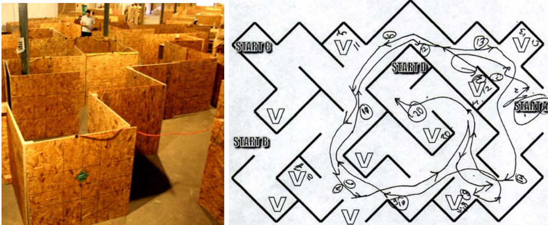
Figure 4-4: The robot operated in the NIST USAR arena (left) while experimenters uses ground truth maps (right) to record specific incidents. In the ground truth map, “Start” symbols represent the four possible starting points, “V” represents a victim location, lines represent the robot path, and circled numbers represent collisions with the arena walls.
