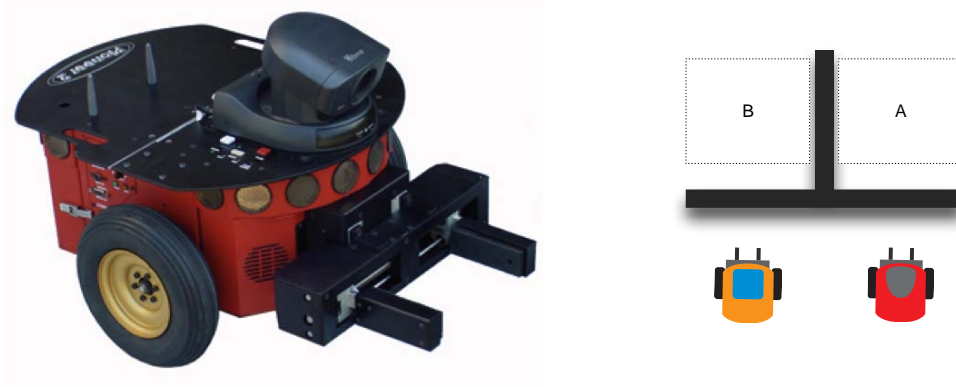
Figure 7-2: Participants were presented with a physical ActiveMedia Pioneer 2Dx robot (left) that was iconically depicted in the experiment slides (right).
