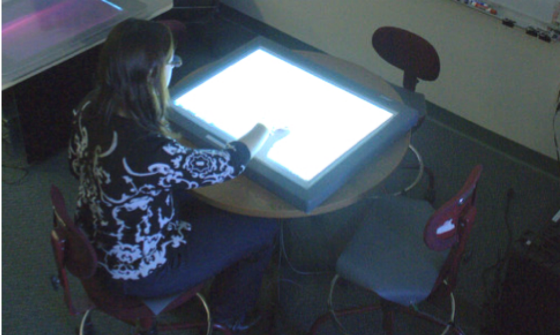
Figure 7-1: Participants were seated in front of a Mitsubishi DiamondTouch fastened to a round table where they provided gestures on a static front projected image.
