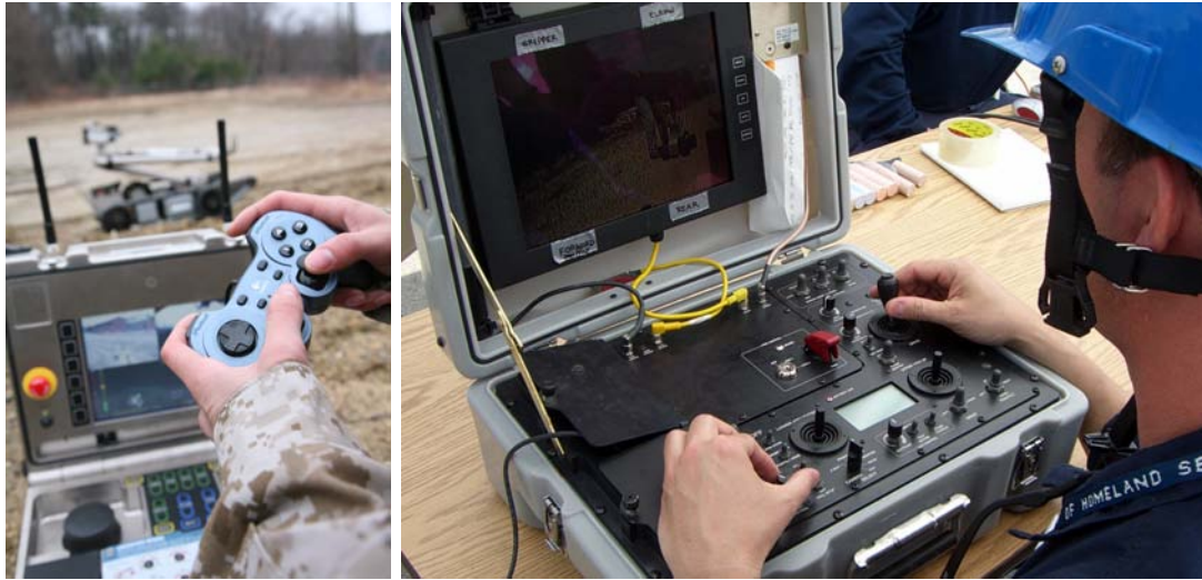
Figure 5-1: The iRobot® Packbot® Hand Controller (left front) is an adapted Sony Playstation® style controller. The Packbot® EOD Operator Control Unit (left rear) places six degrees of freedom on each hand, requiring the operator to manage 12 degrees of freedom and 12 context sensitive push buttons for typical operation. The Foster Miller TALON robot controller (right) is operated through three two degree of freedom joysticks and a large array of switches, selectors, and dials. (Photos courtesy of iRobot Corporation and the National Institute of Standards and Technology.)
