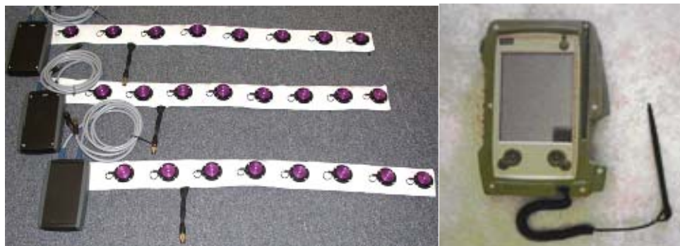
Figure 31. Left: Tactile display belt components with Tractor Components Box (TCB). Each box includes a wireless Bluetooth receiver and the controlling circuitry. Right: Advanced robotics controller (lightweight) PDA that remotely sends the selected signal to the TCB to trigger the tactile message (Developed by Massachusetts Institute of Technology (MIT).
