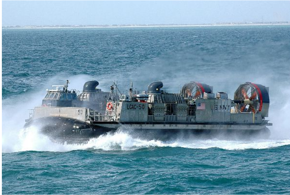
Figure 1. Landing Craft Air Cushion (LCAC) transiting alongside its amphibious transport dock ship (U.S. Navy, 2009a)
