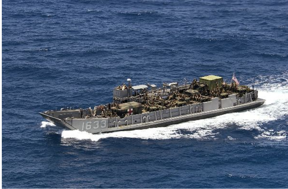
Figure 2. A Landing Craft Utility (LCU) heads to the beach during amphibious assault training. (U.S. Navy, 2009b)
