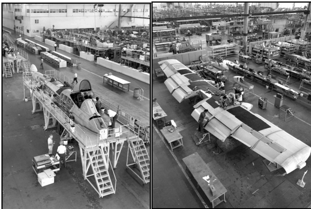
Figure 19. A-10 Fuselage and Wing Production
