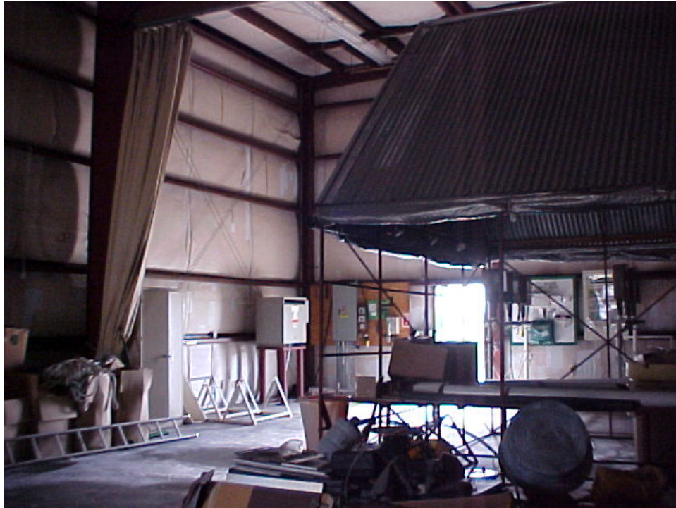
Photograph 51: Additional view of Payload Service Building #003 interior. Roofed structure was used to perform maintenance on the balloon while outside. It was lifted by crane into position.
