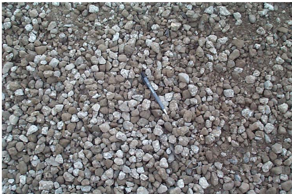
Figure 9. Finished recycled concrete aggregate.
