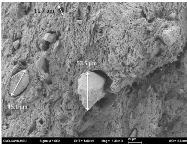
Figure 11: SEM image of fracture surface from room temperature tension at 0.001/s.
