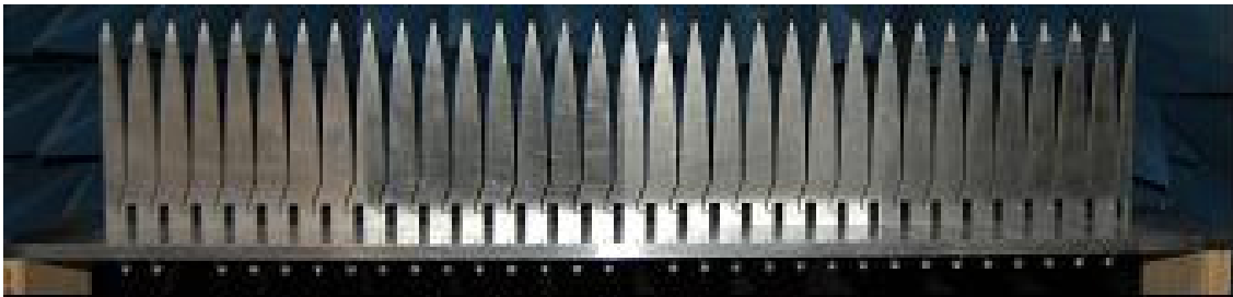
Fig. 2. 32-element linear array of flared notches. The array is constructed from modular sub-arrays of 8 elements.
