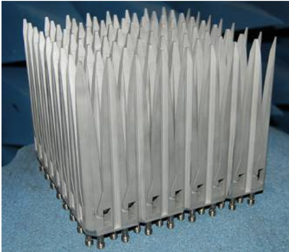
Fig. 3. Assembled 8x8 dual-polarized planar array of flared-notches; 128 total ports, 64 in each polarization. The array is modular and can mate in any direction with arrays of the same size to create larger arrays.
