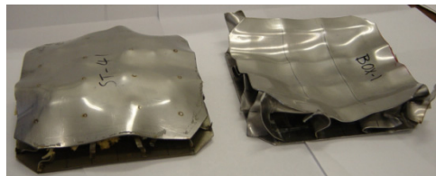
b) Deformed samples after blast tube testing
