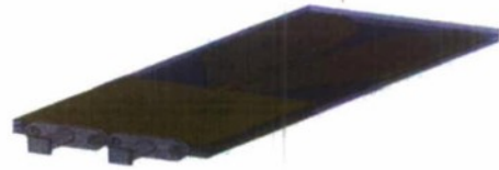
Figure 6 – Ultra-low cross-polarization tapered slot Antenna with embedded balun network.
