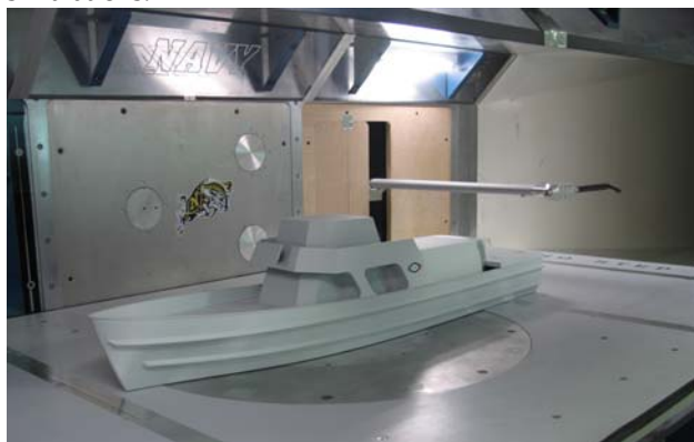
Figure 7. YP hull and basic superstructure in USNA large wind tunnel.
