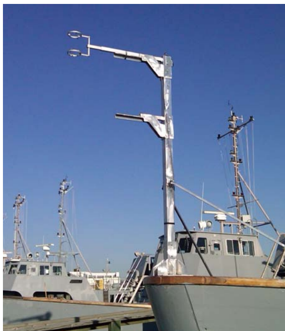
Figure 6. Bow mounted reference anemometer.
