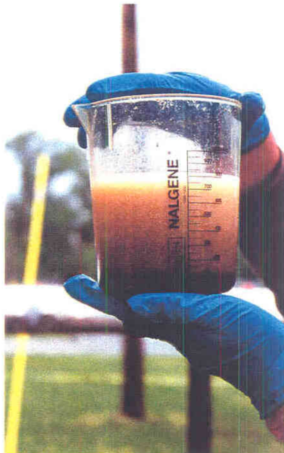
Top and Bottom - Free-phase DNAPL collected during the SEAR demonstration
