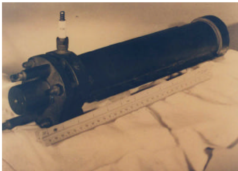
A JATO rocket engine, about 18 inches long.
