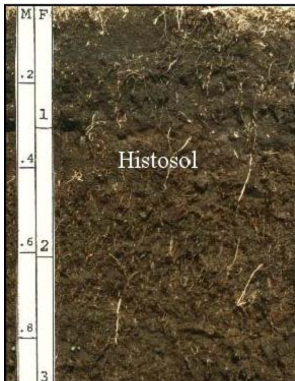
Figure 6. Example of a Histosol, in which muck (sapric soil material) is greater than 3 ft (0.9 m) thick.
